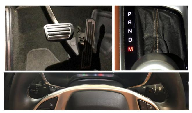
Starting in the upper left corner, you see the brake and gas peddles, the controls for acceleration or deceleration. Then on the right the row of "direction", either **P**arked, **R**everse, **N**eutral (ambivalence), **D**rive and finally and at the center of this discussion **M**ANUAL.
